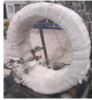
Figure 6 – Thermally insulated coil with ceramic fiber tape.
