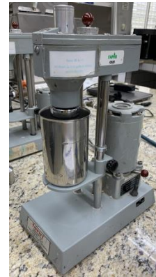
Figure 4 – Fann Viscometer model 35A (Fann Instruments).
