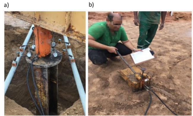
Figure 9 – a) Monometer b) Pump (helps load application).
