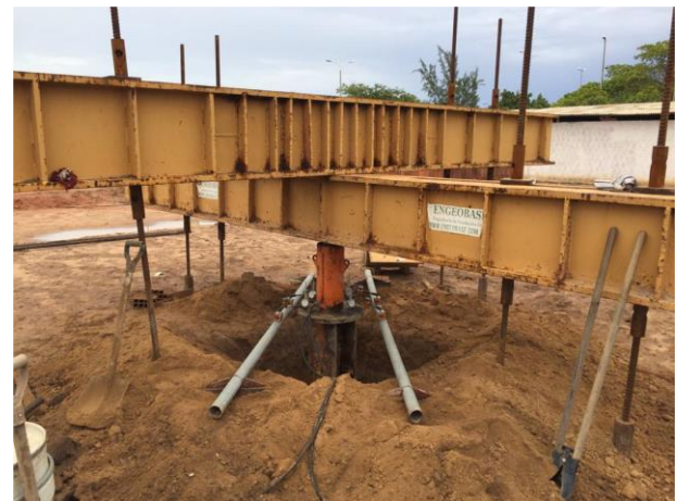
Figure 10 – System test structure.
