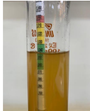
Figure 7 – Density test with the hydrometer.
