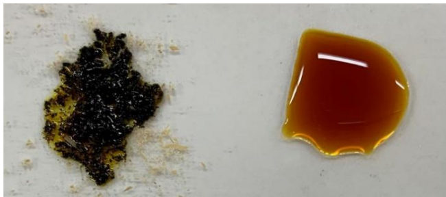
Figure 6 – Iodine test, on the left with reaction, on the right without reaction.
