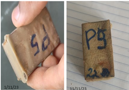
Figure 26 – Test body P5 before (left) and after (right) being completely buried (2x3x5cm).
