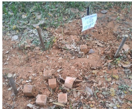
Figure 21 – Buried test bodies.
