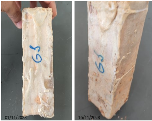
Figure 24- Test body G1 before (left) and after (right) being partially buried (5x5x15cm).
