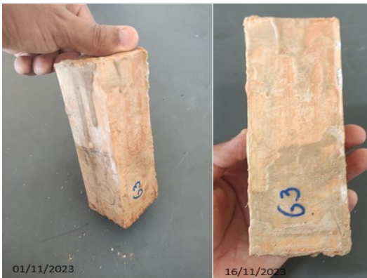
Figure 25- Test body G3 before (left) and after (right) being partially buried (5x5x15cm).
