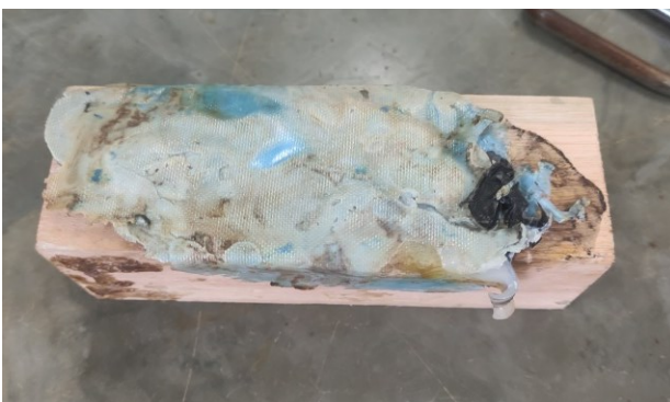
Figure 17 - Test body after molding with melted PET.
