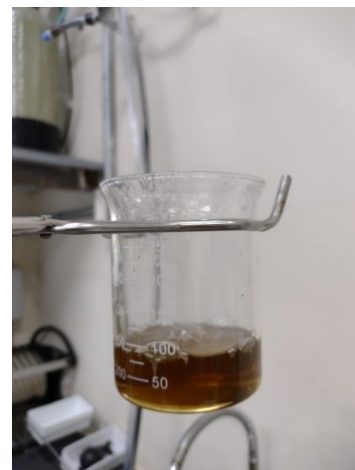
Figure 18 – Plastic resin obtained by heating glycerin with PET 1.
