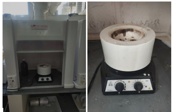
Figure 10 – Fume hood and heating blankets.
